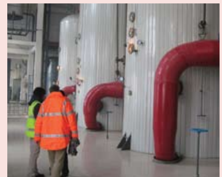
Multiple effect evaporators at the BoTian Sugar factory in Zhangbei, northern China.
