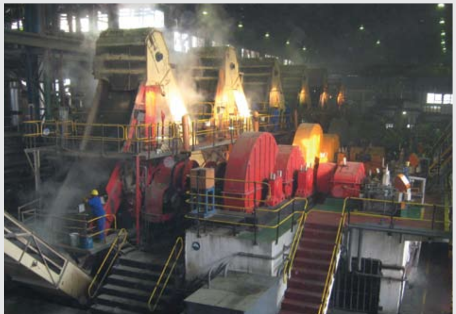
The sugar extraction section of the Maragra Mill in Mozambique.
